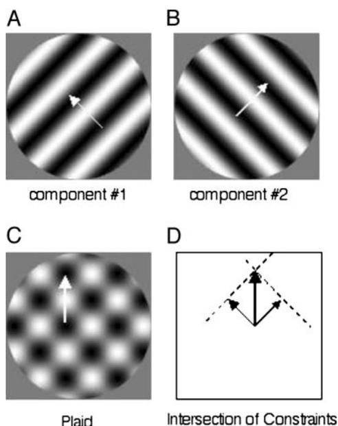
FIG. 1. A–C: plaid pattern and its constituent gratings. D: intersection of constraints computation. Gratings A and B add together to form plaid C. Each grating has direction and speed of motion indicated by white arrows. Plaid C has direction and speed of motion that can be calculated from intersection of constraints (IOC). See text for further explanation.
